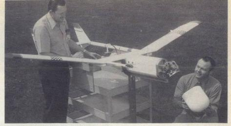
Melpar's E-45 mini-RPV has a 95 inch wing span and has a takeoff weight of 45 lbs. It uses a two HP, one cylinder engine and has an endurance of four to five hours. It's shown here with gimbaled TV reconnaissance camera in its nose but it has also been flight tested as a homing Kamakazi vehicle, with a D/F receiver as a payload.
