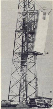
1. Rectenna array consists of 17 subarrays in a 3 x 6 matrix. Each subarray contains 270 dipole antennas and diode rectifiers. The standard gain horn at lower right of array is used for power calibration. The rectenna is inclined at 7 degrees so the microwave beam doesn't reflect off the ground.
