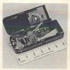
1. The 94 GHz radar developed for Coast Guard tests (a) uses a 24-inch parabolic dish with a gain of 52 dB. Circuitry is housed in the  $11 \times 4.5 \times 4$  inch box attached to the antenna's frame. Scarcely larger than a flashlight, the hand-held unit shown on the right (b) illustrates how small a 94 GHz radar can be.
