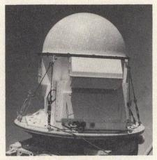
3. Passive phase shifters are visible in the hemispherical dome of this C-band feasibility model. Production models may use printed-circuit elements glued to the inside of a honeycomb dome.
