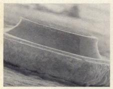
5. Scanning electron photomicrograph shows an Impatt mesa with plated gold heat sink. Silver and copper are also used and provides slightly lower thermal resistances.
