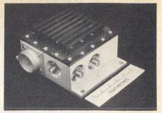
9. MIC paramp developed by Marconi provides a 200°K noise temperature at 7 GHz.
