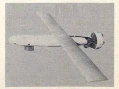
3. Acquare mini-RPV weighs 150 lbs and uses a 12 HP single cylinder Mc Cullough engine. Its payload includes a stabilized TV sensor plus laser designator derived from Aeronutronic Ford's Praerie II.
