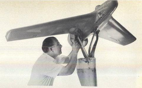
4. Half-size model of Aquila mini-RPV is shown here in wind-tunnel tests. The final delta wing version will be 6 ft. long with a wing span of 11.9 ft and total weight including
