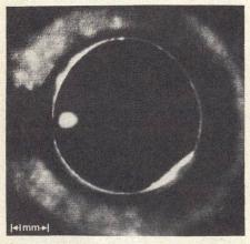
1. Photo of a single (1/30 inch diameter) electron-hole drop was obtained by illuminating a Ge crystal with a laser on one side and focusing an infra-red sensitive TV vidicon on the opposite side. The Ge crystal disk in which the drop forms measure 4 mm in diameter and 1.4 mm thick. Laser pump level is 80 mW at about 5000 Å. The outline of the stressing screw is seen on the left.
