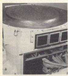
1. A simple, planar array can provide greater than hemispherical coverage when capped with a dielectrically-loaded lens.
