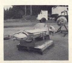
2. Acquare mini-RPV, in stowed position before loading in fiberglass pod, has its wings folded atop fuse-lage so it can fit. After it is dropped, explosive bolts release RPV from the pod and its wings pivot and lock in place for flight.
